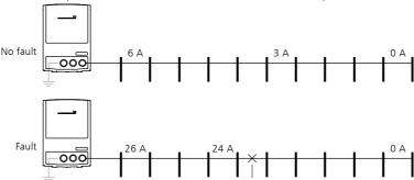
3 Move backwards in the direction of the highest reading to locate the fault.
